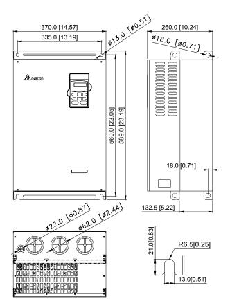
Frame E1: VFD300B23A, VFD370B23A, VFD550B43C/53A, VFD750B43C/53A
