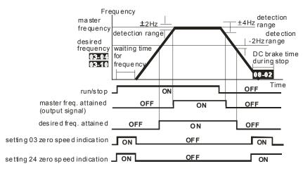
output timing chart of multiple function terminals when setting to frequency attained or zero speed indication
