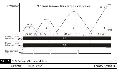
This parameter controls the direction of motion for the Multi-Step Speeds Pr.05-00 to Pr.05-14 during PLC mode. All other direction commands are invalid during the PLC mode.
