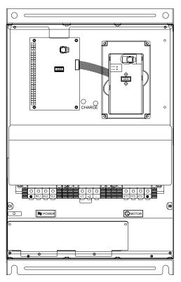
Control Terminal Torque: 4Kgf-cm (3 in-lbf) Wire: 12-24 AWG (3.3-0.2 mm<sup>2</sup>)
