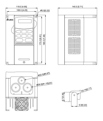
Frame B: VFD022B21A, VFD037B23A/43A/53A
