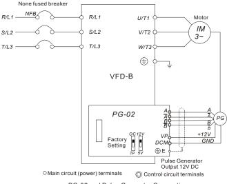
PG-02 and Pulse Generator Connections
