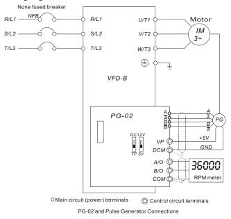
2. Basic Wiring Diagram with RPM Meter Attached.
