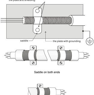
Remove any paint on metal saddle for good ground contact with the plate and shielding.
