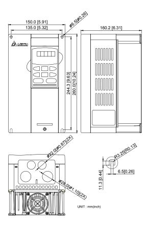
Frame C: VFD055B23A/43A/53A, VFD075B23A/43A/53A, VFD110B23A/43A/53A
