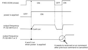
The Line Start Lockout feature does not guarantee that the motor will never start under this condition. It is possible the motor may be set in motion by a malfunctioning switch.
