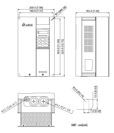
Frame D: VFD150B23A/43A/53A, VFD185B23A/43A/53A, VFD220B23A/43A/53A
