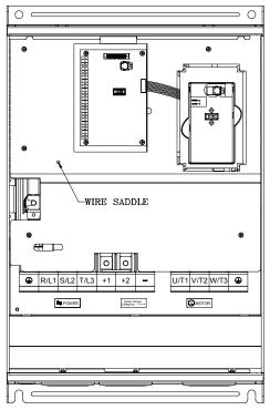
Control Terminal Torque: 4Kgf-cm (3 in-lbf) Wire: 12-24 AWG (3.3-0.2 mm<sup>2</sup>)
