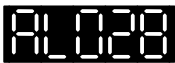
AL028 : The encoder is over voltage or the internal of the encoder is in error
