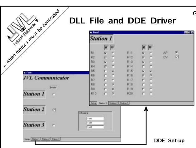
JVL's DLL (Dynamic Linked Library) file and DDE (Dynamic Data Exchange) driver make it possible to develop and use Windows software with JVL's AC and DC Servo Motor Controllers and Servo/Step Motor Indexers.
