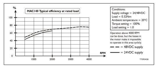
The power consumption for the internal circuitry (microprocessor etc.) is typically < 3.5W. In the speed range from 0 to 500 RPM this internal power consumption starts to be a dominant part of the total power consumption which explains that the efficiency starts to be lower.
