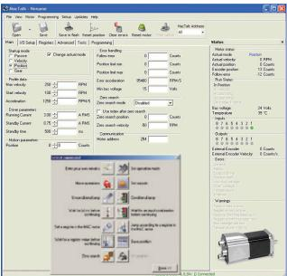
The MacTalk software is the main interface for setting up the QuickStep motor for a specific application.
