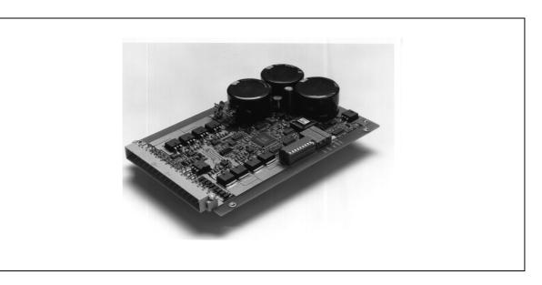
Type PA0076 is an advanced multifunction step motor driver that can be controlled either by step pulses from an external source or by the internal step generator.
