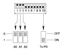
Baud Rates of 110 to 9600 Baud can be selected for communication using the Controller's RS232C interface. The Baud Rate is configured by setting 3 DIP switches, as shown in the following table.
