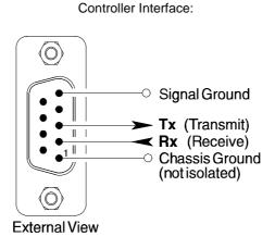
For communication with the Controller via a PC, the interface connections are illustrated in the following figures.
