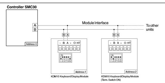
Controllers Type SMC30 can be connected to external modules such as a, input/output-module, keyboard/display-module etc.
