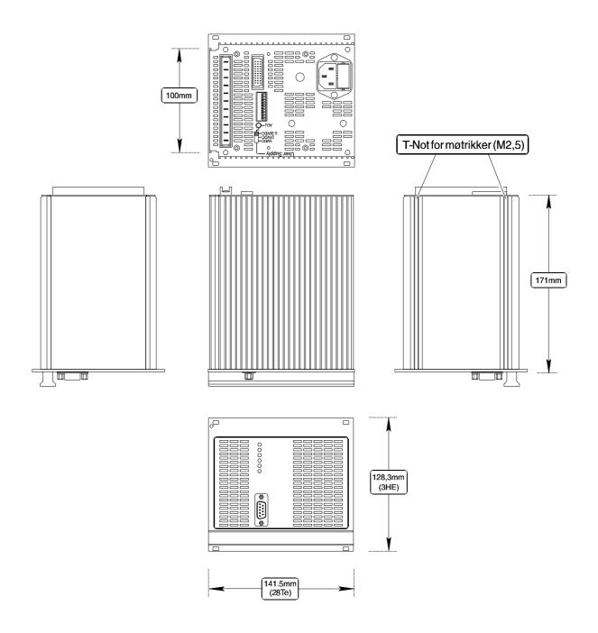
If the Controller is mounted in a closed cabinet, a ventilation fan or other form of cooling should be installed. The Controller is however protected against overheating by a built-in thermo-switch which disconnects the driver stages at a temperature of approximately 80 °C.
