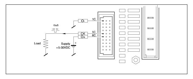
For use in motion-control systems where several step motors are operated synchronously, Controller SMC30 is equipped with a step-pulse Clock Output which outputs a voltage pulse for each motor step. The Clock Output can also be used for connection of a counter or similar equipment which is used to track motor position.
