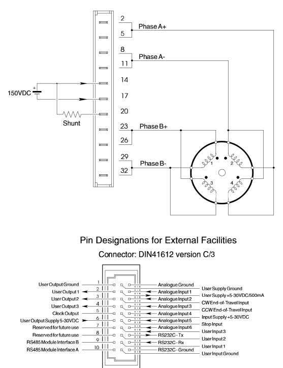
The Controller Interface uses the widespread RS232C standard, which provides a great degree of flexibility since all Personal Computers and standard terminals have provision for using this communication standard. For operation of the Controller via an RS232C interface, the 3 standard RS232 connections Rx, Tx and Ground are used.
