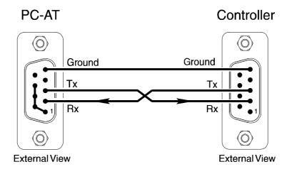
Connection between the Controller and an IBM XT/PS2 or compatible :
