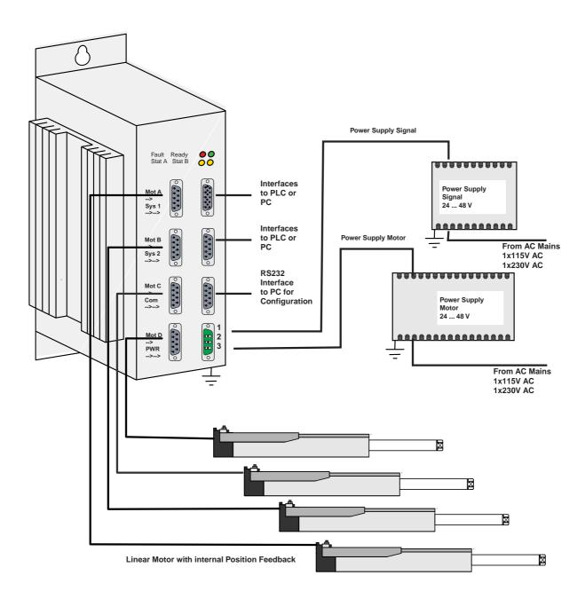
Complete E400 Controller based system (E100 and E200 controllers will only drive one respectively two motors). Power Supply for Signal and Motor may be the same device (see later).
