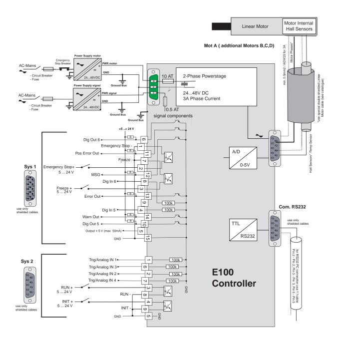
Picture shows typical wiring of a single axes controller. Multiple axes controller will have additional motor connectors.
