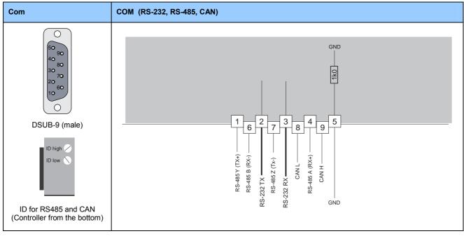
9.6kBaud, use 1:1 connection cable to PC RS232: RS485 and CAN needs external termination (see manual)
