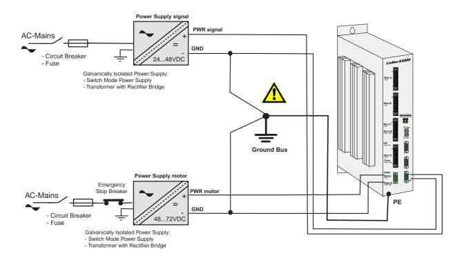
Instead of two separated power supplies it may be possible to use only one power supply of 48V if there is no need to control the signal power supply (logical devices of the controller) and the power supply of the powerstage for the motors independently (see safety rules of the application).
