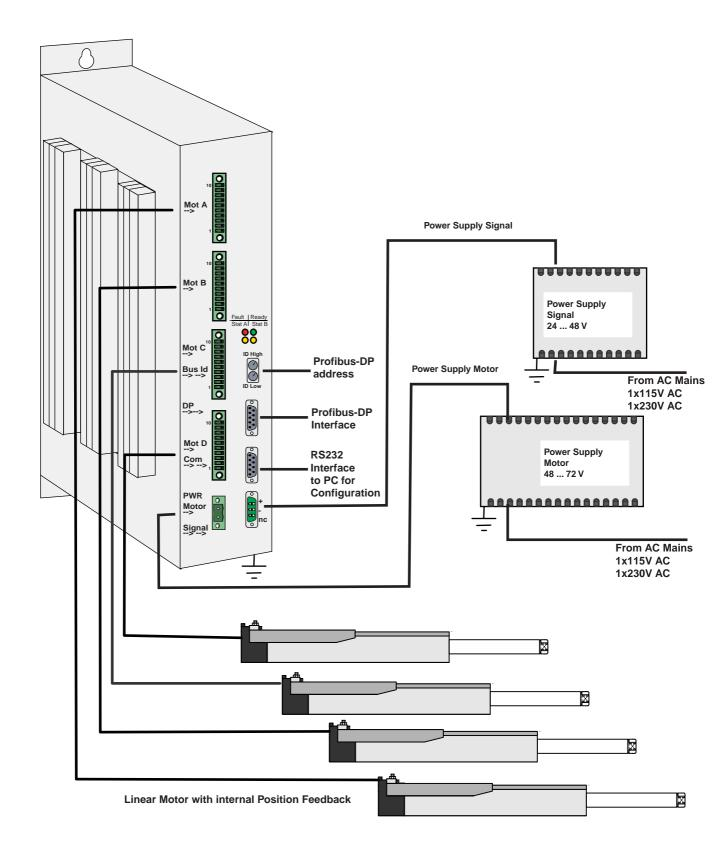
Complete E4030 Controller based system (E1030 and E2030 controllers will only drive one respectively two motors). Power Supply for Signal and Motor may be the same device (see later).
