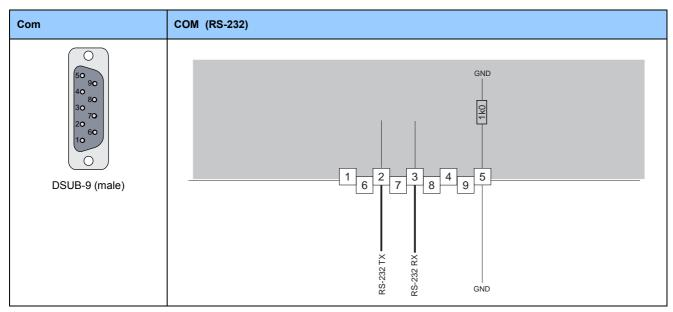
RS232: 9.6kBaud, use 1:1 connection cable to PC
