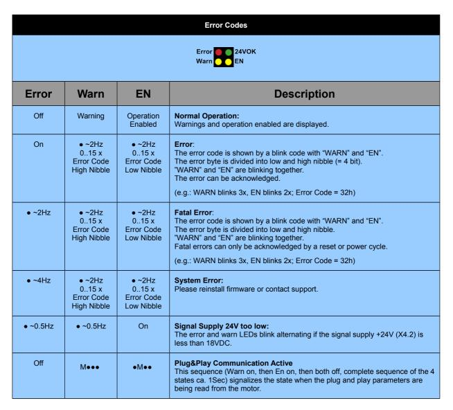
The meaning of the error codes can be found in the Usermanual\_MotionCtrl\_Software\_SG5 and the user manual of the installed interface software. These documents are provided together with LinMot-Talk configuration software and can be downloaded from <a href="https://www.linmot.com">www.linmot.com</a>.
