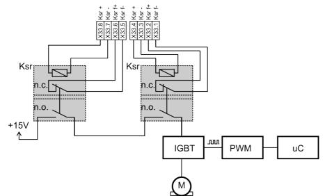
To enable the -1S drives both relays have to be switched on. Minimal wiring:
