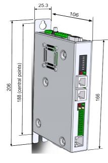
C12X0-XX-XX-0S mounting points for M5 screws all dimensions in mm
