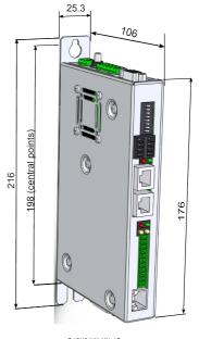
C12X0-XX-XX-1S mounting points for M5 screws all dimensions in mm
