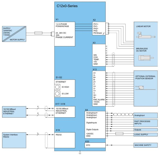
Typical Servo System C12x0-XX: Servo Drive, Motor and Power Supply.
