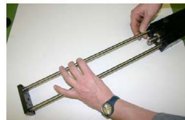
Move lubricated (ball bearing grease eg.SKF LGMT2) Guide Unit slowly into Guide
