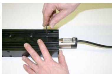
Tighten stator clamping screws ( torque: 200 Ncm (1.47 ft lbs)).
