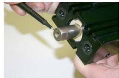
End of the slider with serial number must be on the forward end as shown!
