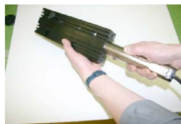
Insert Stator (clamping parts may have to be moved)
