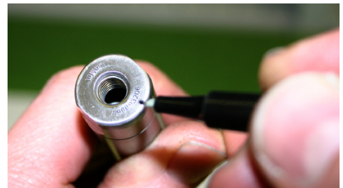
End of the slider with lasered serial number
