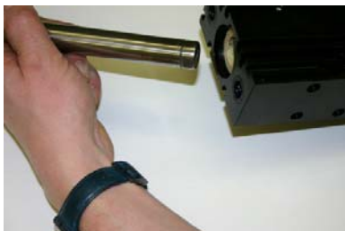
Place lubricated (LinMot grease LU02) Slider into the Stator (End without serial number)
