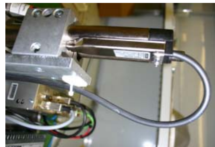
Maintain minimum bending radius of 25 mm
