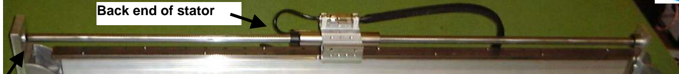
Fixed Slider End (Ball and Socket Mounting) Principle of a Moving Stator application Floating Bearing
