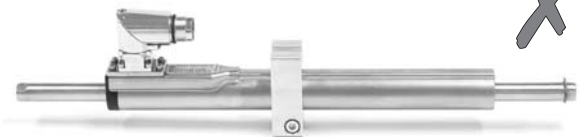
Incorrect: Small mounting surface area prevents proper cooling of the linear motor.
