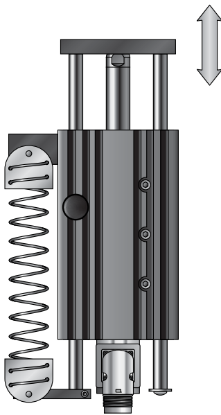
Weight compensation with mechanical spring
