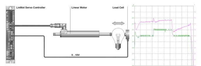
Servo drives E1100, E1200, E1400 or B1100 with force control technology function. The force applied to the object is generated by the linear motor and measured in the load cell. The applied force measured in the load cell is directly fed back to the servo drive.
