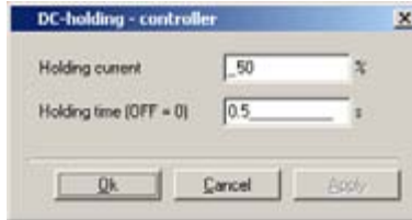
Fig. 8.9 Function mask DC holding current controller
