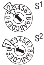
Figure 2.3 Coding switches for PROFIBUS address
