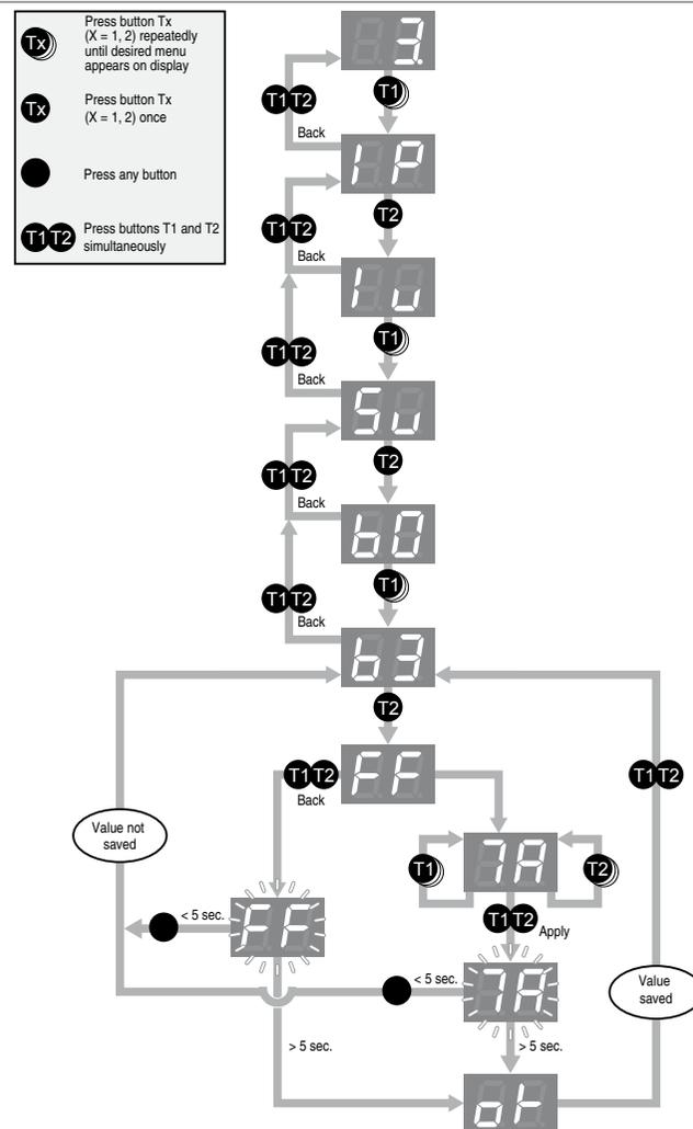
Figure 4.2 Example configuration of subnet mask
