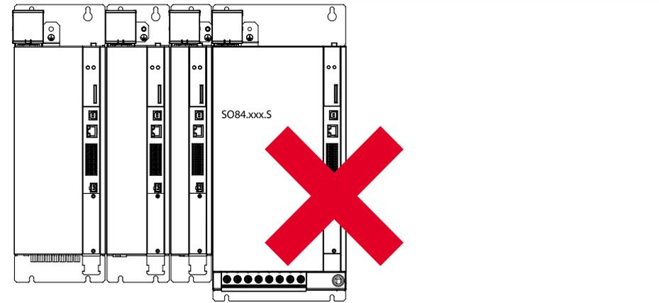
Figure 2.11 Example of an **impermissible** layout: Arrangement of ServoOne DC axis controllers in ascending order of size
