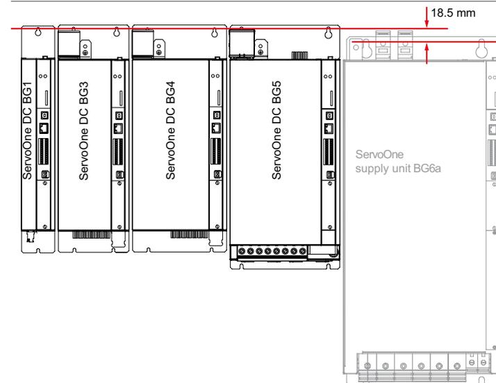
Figure 2.2 Row of air-cooled DC axis controllers adjacent to supply unit BG6a (example)
