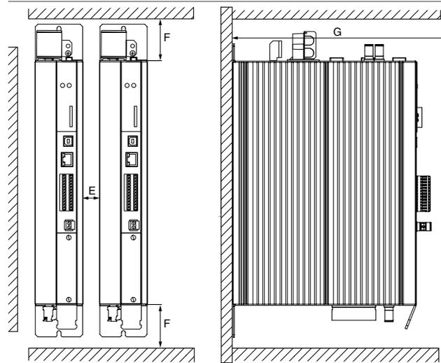
Figure 2.4 Mounting clearance, wall-mounted housing
