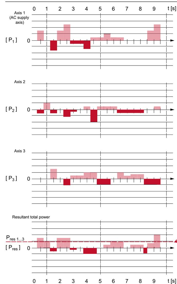
Figure A.4 Time/power graph with servocontroller as supply
