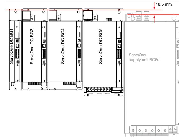
Figure 2.6 Row of liquid-cooled DC axis controllers adjacent to supply unit BG6a (example)
