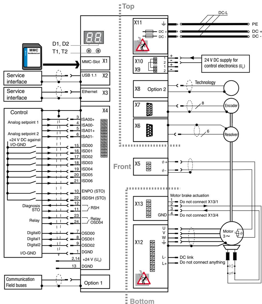
Figure 3.2 Connection diagram, BG1 to BG4
