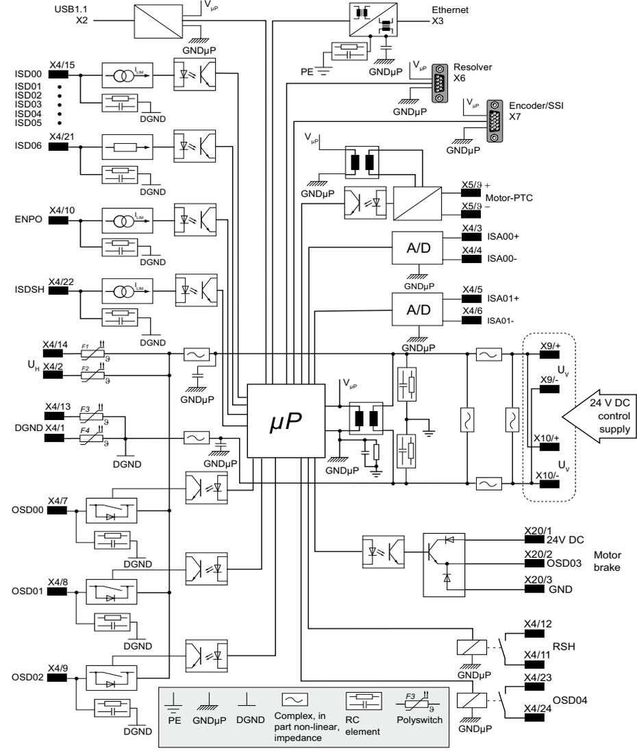
Figure 3.7 Electrical isolation method, BG5 and BG6a
