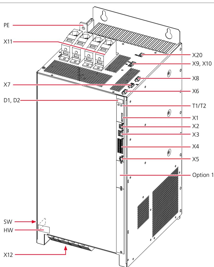
Figure 3.4 Layout, BG6a (without shields)
