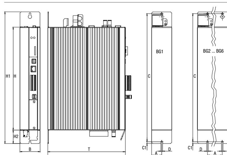
Figure 2.3 Dimensional drawing, wall-mounted housing
