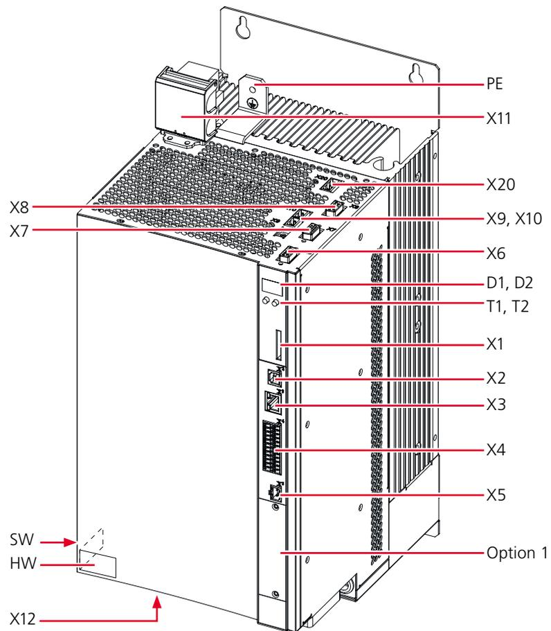
Figure 3.3 Layout, BG5 (without shields)
