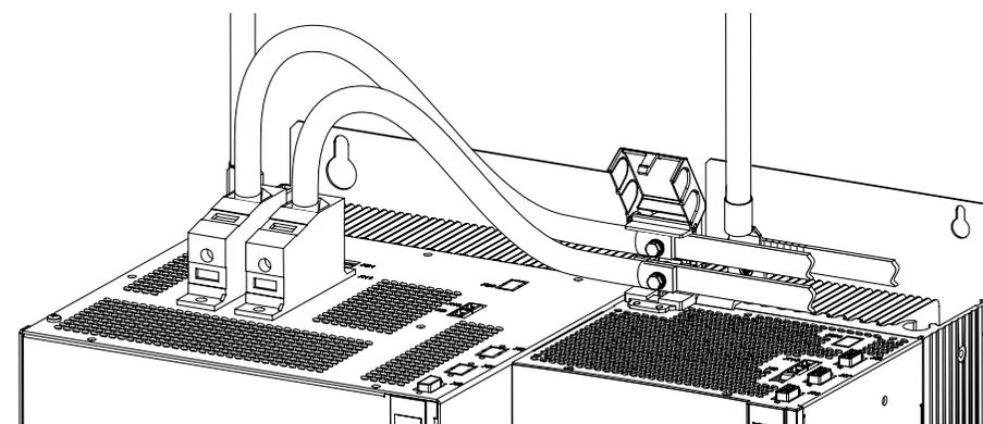
Figure 3.10 Detail: BG6a DC power supply connection to smaller DC axis controllers
