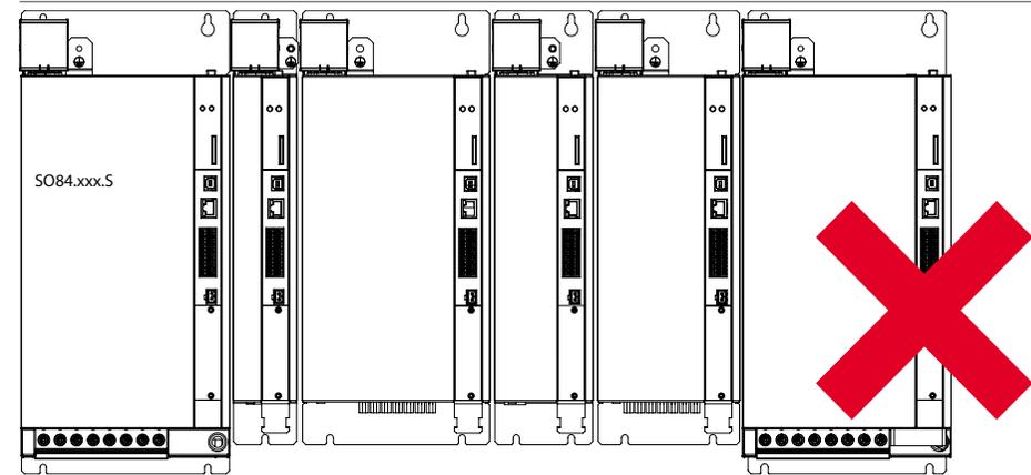
Figure 2.12 Example of an **impermissible** layout: Arrangement of ServoOne DC axis controllers in ascending and descending order of size
