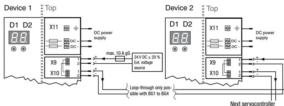
Figure 3.8 Connection of control supply
