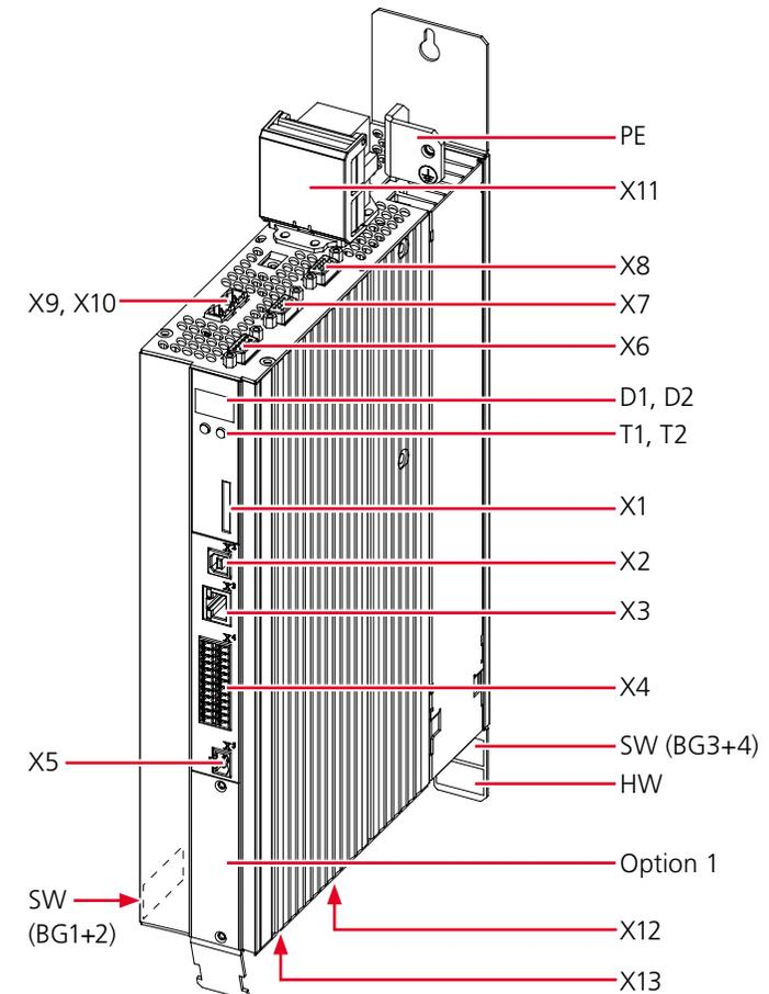
Figure 3.1 Layout, BG1 to BG4 (here: BG1)
