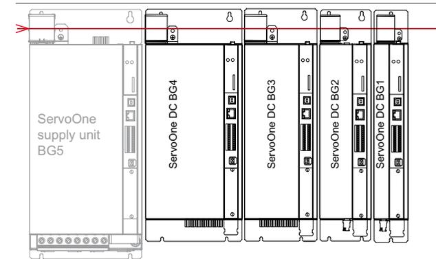
Figure 2.5 Row of liquid-cooled DC axis controllers adjacent to supply unit BG5 (example)
