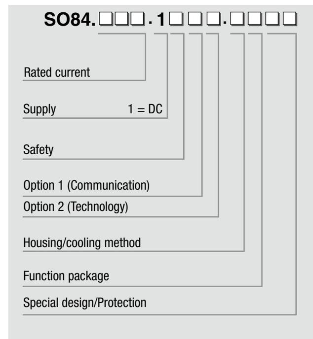
Figure 0.1 Order code – ServoOne multi-axis system DC axis controller
