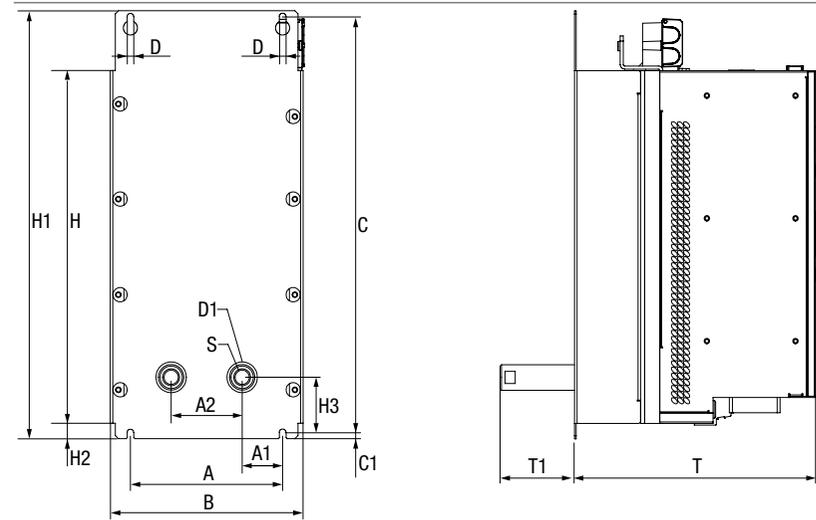
Figure 2.7 Dimensional drawing, liquid-cooled unit
