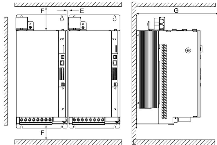
Figure 2.8 Mounting clearance, liquid-cooled unit
