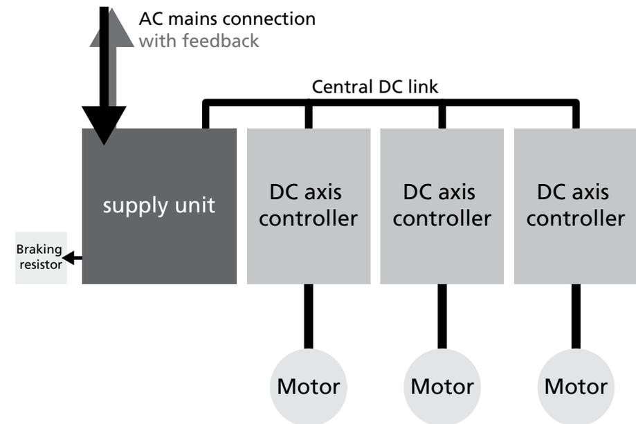
Figure A.1 Block diagram of a multi-axis system with supply unit and mains feedback
