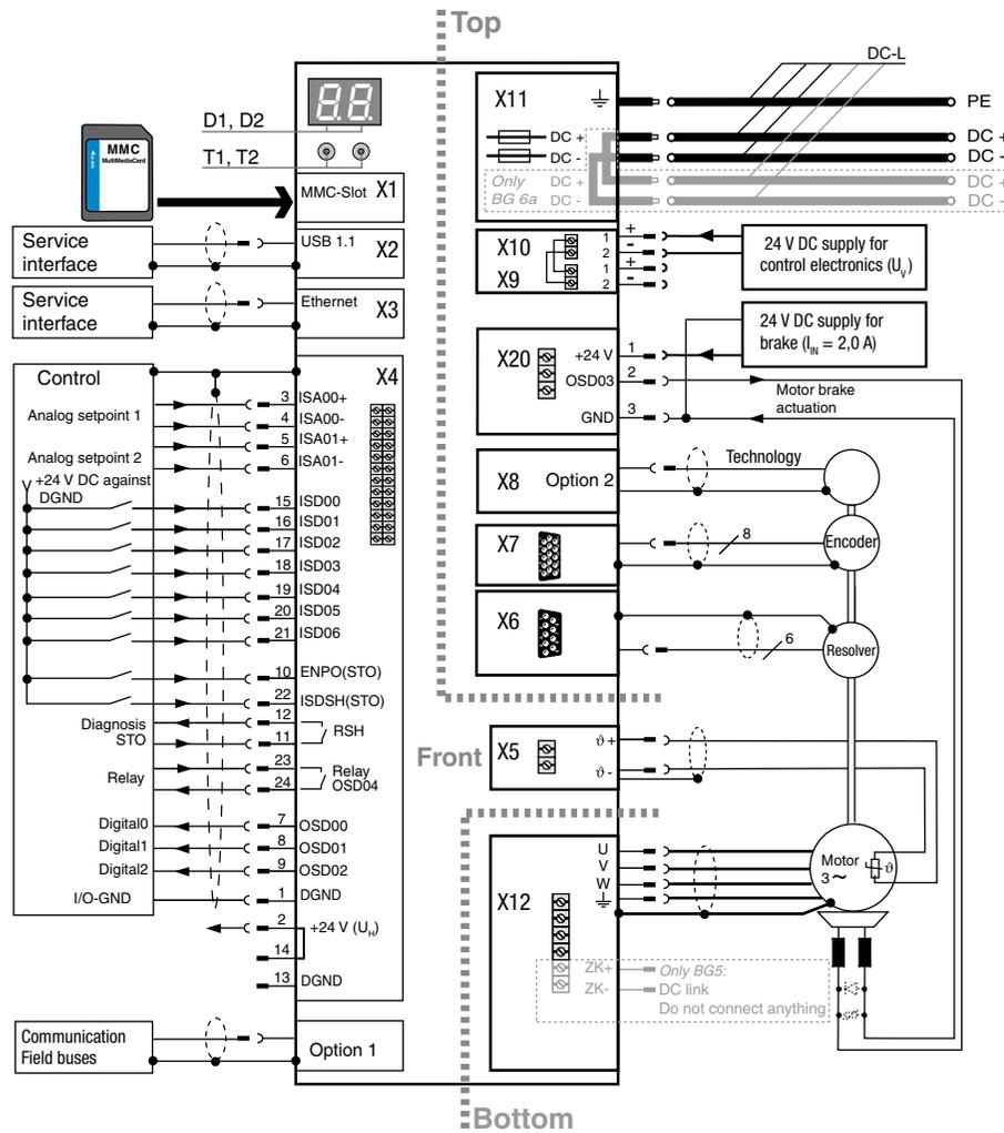
Figure 3.5 Connection diagram, BG5 and BG6a
