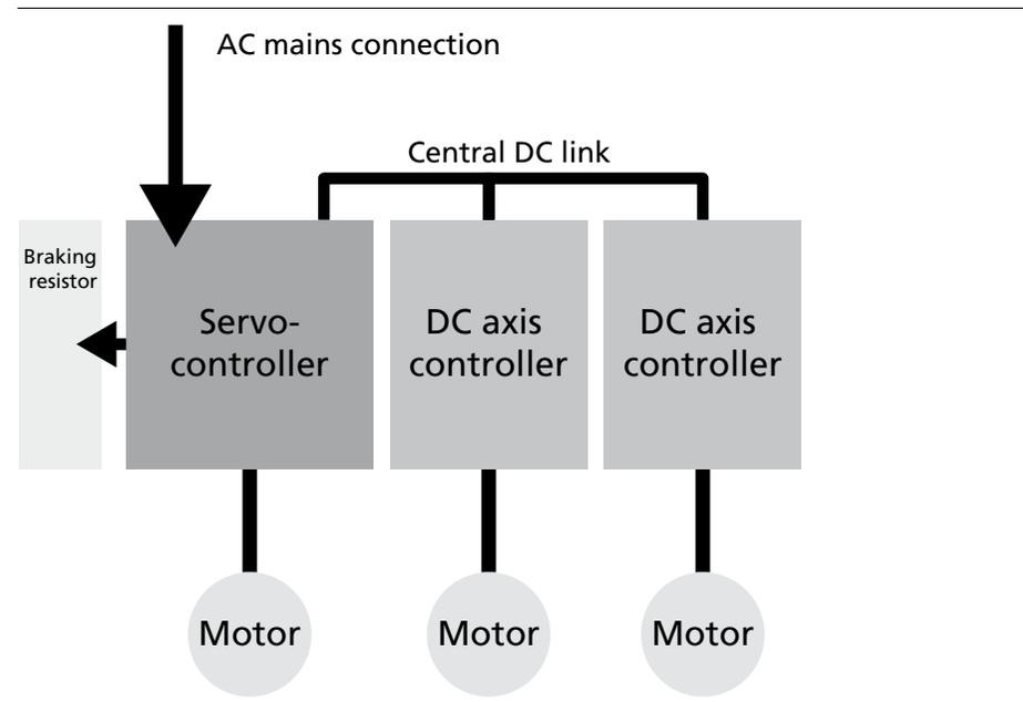
Figure A.2 Block diagram of a multi-axis system with servocontroller as supply
