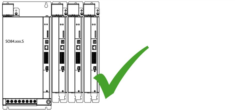
Figure 2.9 Example of a permissible layout: Arrangement of ServoOne DC axis controllers of same size on one side of the supply unit
