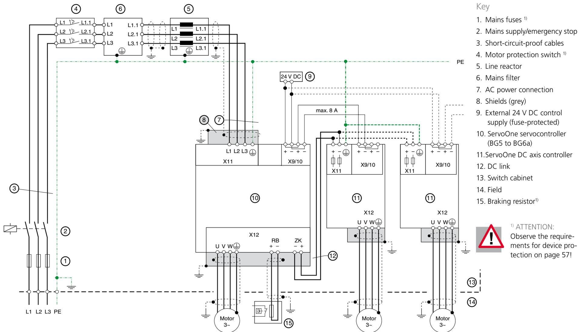
Figure 7.2 Overview - Connection diagram for operation with supply by servocontroller (BG5 to BG6a)
