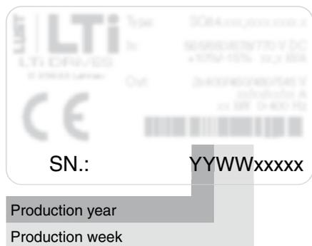
Figure 0.2 Hardware rating plate – ServoOne multi-axis system DC axis controller
