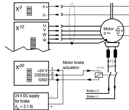
Figure 3.14 Connection of motors BG5 and BG6a
