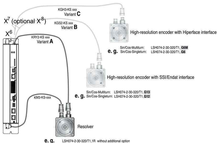
Figure 3.12 Matching motor/encoder cable
