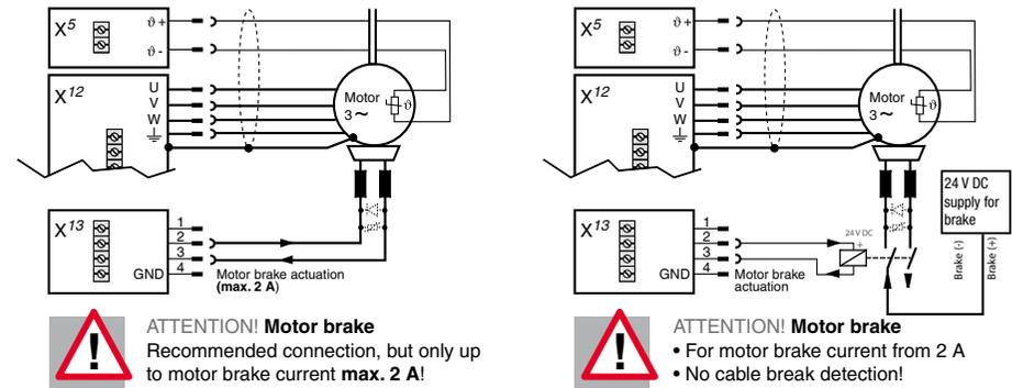
Figure 3.13 Connection options of motors BG1 to BG4
