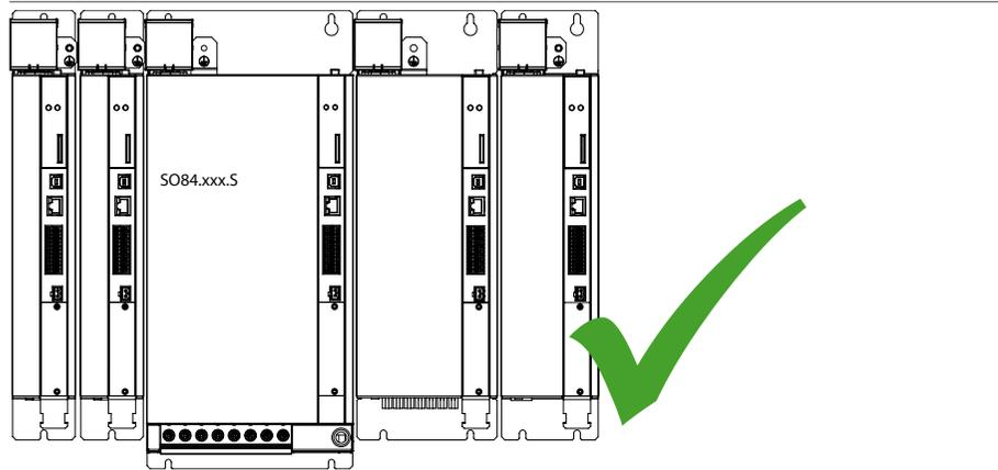
Figure 2.10 Example of a permissible layout: Arrangement of ServoOne DC axis controllers of same size and in descending order of size on both sides of the supply unit respectively
