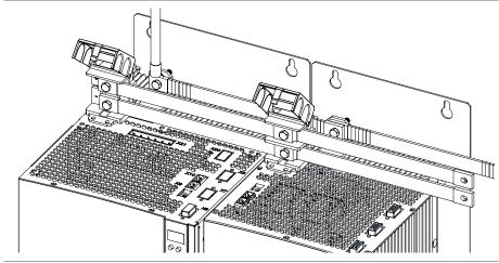
Figure 3.9 Detail: DC power supply connection, BG5
