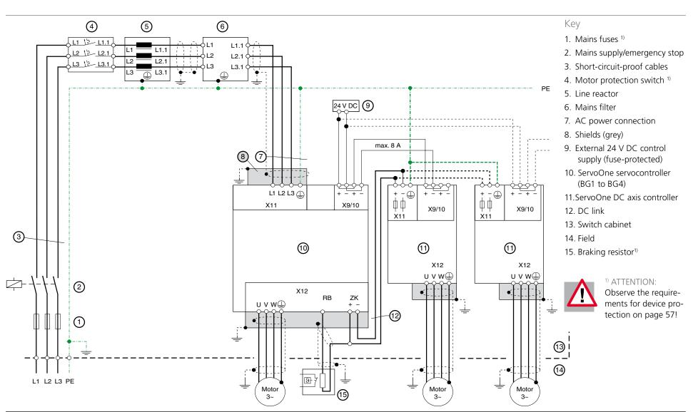
Figure 7.1 Overview - Connection diagram for operation with supply by servocontroller (BG1 to BG4)
