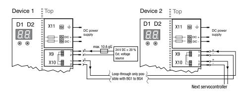
Figure 3.8 Connection of control supply
