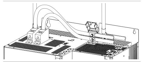
Figure 3.10 Detail: BG6a DC power supply connection to smaller DC axis controllers
