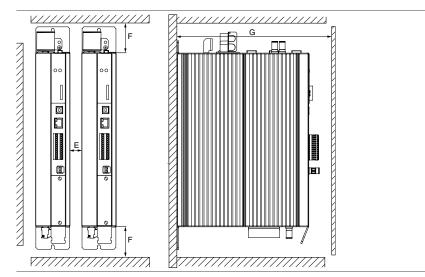
Figure 2.4 Mounting clearance, wall-mounted housing
