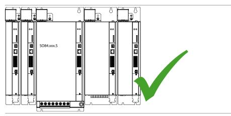
Figure 2.10 Example of a permissible layout: Arrangement of ServoOne DC axis controllers of same size and in descending order of size on both sides of the supply unit respectively
