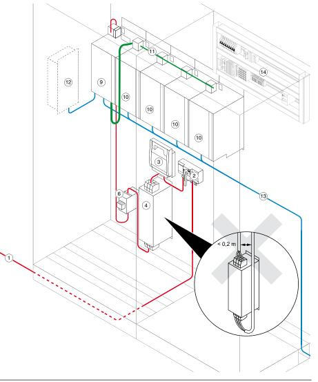
Figure 7.4 Switch cabinet layout, multi-axis system with supply by servocontroller (as from BG5)
