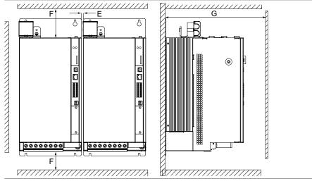
Figure 2.8 Mounting clearance, liquid-cooled unit
