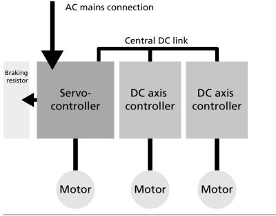
Figure A.2 Block diagram of a multi-axis system with servocontroller as supply
