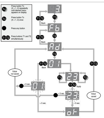
Figure 4.3 Example configuration of field bus address
