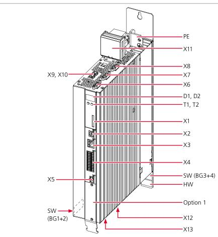
Figure 3.1 Layout, BG1 to BG4 (here: BG1)
