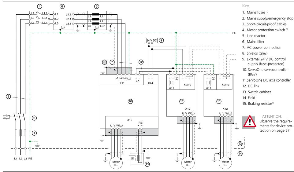
Figure 7.3 Overview - Connection diagram for operation with supply by servocontroller (BG7)
