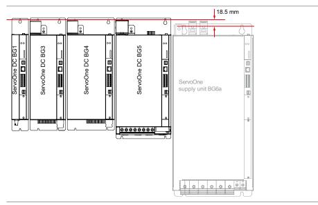
Figure 2.2 Row of air-cooled DC axis controllers adjacent to supply unit BG6a (example)
