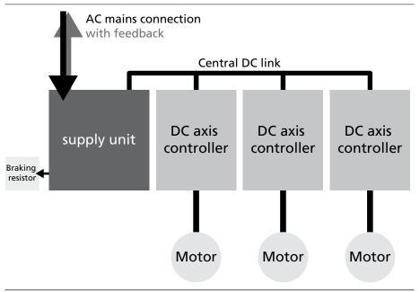
Figure A.1 Block diagram of a multi-axis system with supply unit and mains feedback
