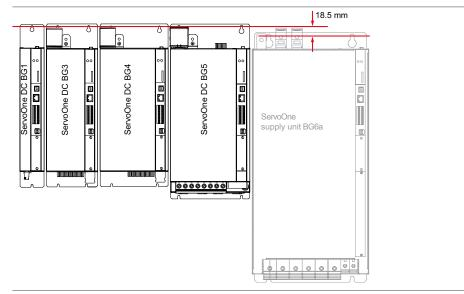
Figure 2.6 Row of liquid-cooled DC axis controllers adjacent to supply unit BG6a (example)
