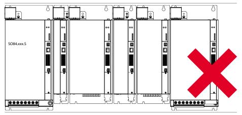
Example of an *impermissible* layout: Arrangement of ServoOne DC axis controllers in ascending and descending order of size Figure 2.12
