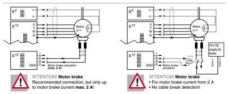
*Figure 3.13* Connection options of motors BG1 to BG4
