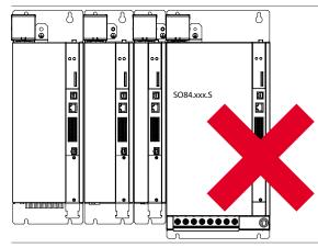
Figure 2.11 Example of an *impermissible* layout: Arrangement of ServoOne DC axis controllers in ascending order of size
