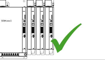
*Figure 2.9 Example of a permissible layout: Arrangement of ServoOne DC axis controllers of same size on one side of the supply unit*
