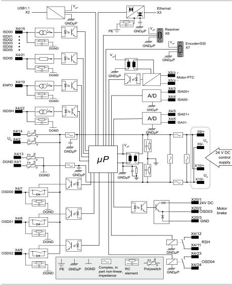
Figure 3.6 Electrical isolation method, BG1 to BG4
