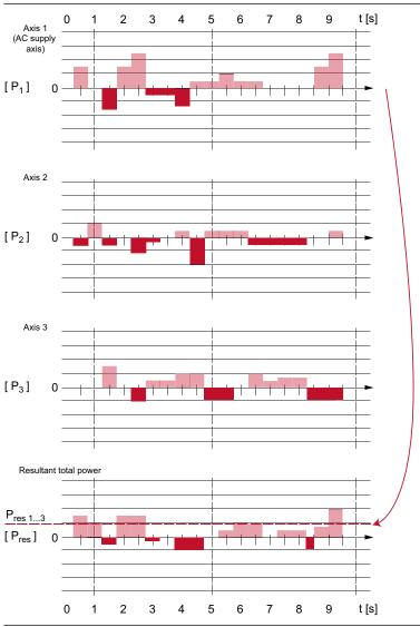
Figure A.4 Time/power graph with servocontroller as supply
