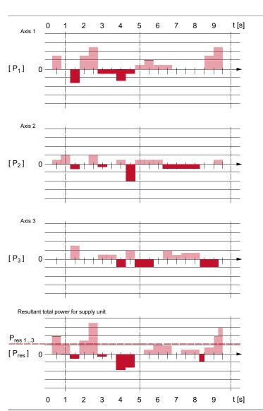
Figure A.3 Time/power graph with supply unit
