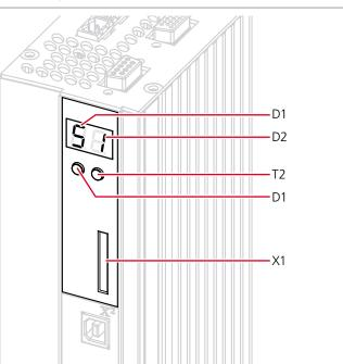
*Figure 4.1 Integrated operator control unit*
