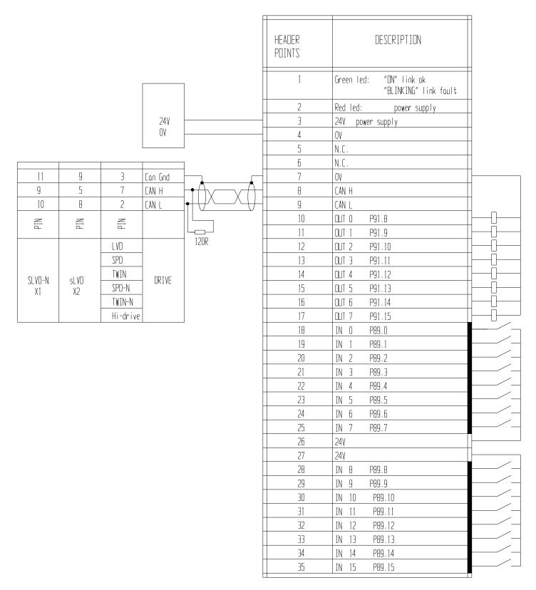
Note: be carefully regarding I/O BOX version! There are two types of I/O BOX: one is compatible only with LVD DRIVE, and another is for. sLVD, SPD, TWIN, SLVD-N, SPD-N, TWIN-N and HID DRIVE.
