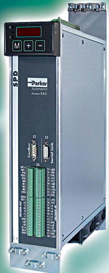
SPD 2-5-8-16-24 2÷25 Arms 230 Vac single/three-phase 380÷480 Vac three-phase
