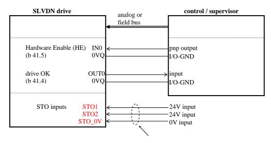
The user must exclude the risk of any short circuit. Cable installation in the cabinet according to the EN directives. The user must insert external fuse for 24VDC supply between the safe disable wiring and the 24V supply. Segregate the wiring in a dedicated raceway or use a shielded wire with grounded shield. The safety function guarantees machine safety only if it is correctly applied in the whole machine safety plant.
