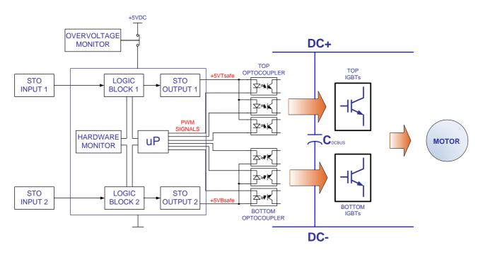
STO function is active low. If the inputs, STO IN 1 and STO IN 2, are high, the output signals, +5VTsafe and +5VBsafe are high (+5V), and the optocouplers that drive top and bottom IGBTs are enabled. If STO IN 1 and STO IN 2 input are low, +5VTsafe and +5VBsafe signals are low and top and bottom optocouplers shutdown.
