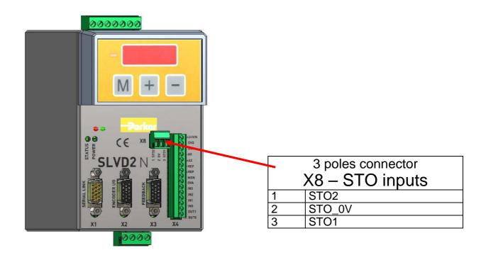
The following diagram shows how to use the safe torque off. They should be considered as a generic reference example. Any specific machine/application design must be analysed.
