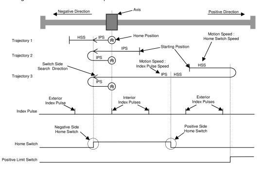
For simplifying diagrams, the trajectory of the switch side search is not explicitly drawn. However, an arrow indicates the direction used to search a switch side. Hence, trajectory 1 of homing method 8 is explained in the following diagram:
