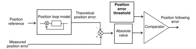
The measured position error value is continuously compared with the theoretical position error given by the position loop model. When the difference is exceeding the **Position error threshold**, the position following error is released. In this configuration, when the position servo loop is adjusted to get the motor position continuously
