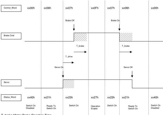
T\_brake Motor Brake Reaction Time
