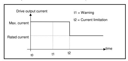
The maximum current duration before warning (t1 - t0) and before limitation at the rated current (t2 - t0) is calculated the same way as in the "Fusing" mode.
