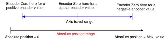
The object 0x312B,1 allows to set the Encoder Zero at the current position:
