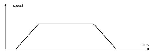
The profile starts as soon as Virtual Master Speed is set with the defined acceleration, and the master signal slows down and stops when Virtual Master Speed is reset at 0. The virtual master output object can be used as master-slave input signal or distributed over CAN bus via PDO.
