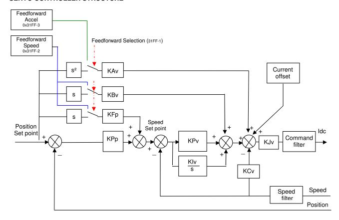
**Speed loop** gains are the most critical adjust because they greatly depend on the mechanical load characteristics (inertias, frictions, coupling stiffness, resonances,...).
