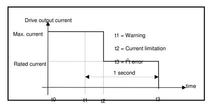
The maximum current duration before release of the warning is depending on the value of the parameters **Rated current** and **Max. current**. This value is calculated as follows:
