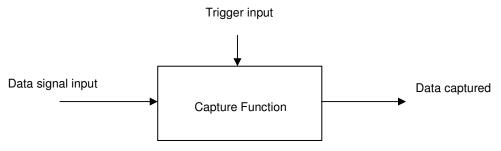
The purpose of the capture function is to latch a data signal (generally position value from a sensor) on a trigger input signal (generally a logic input).
