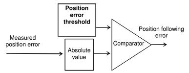
The measured position error value is continuously compared with the **Position error threshold** parameter value. When the measured position error is exceeding the **Position error threshold**, the position following error is released. This configuration is used for applications requiring the smallest possible following error.
