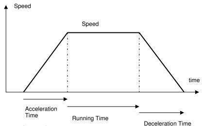
The main parameters of a speed sequence are:
