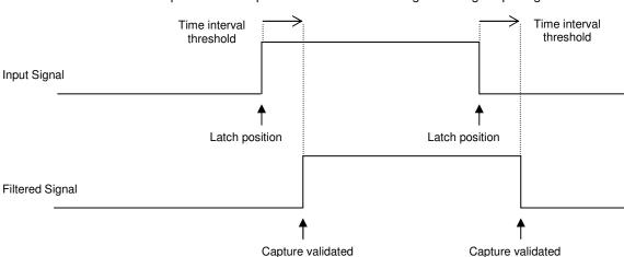
Capture of motor position while motor running with a logic input signal
