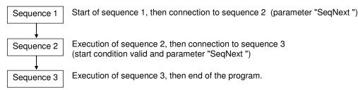
If the execution is starting at sequence 1 and logic input 8 is deactivated, the program will be the following:
