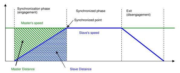
In this coupling mode, the slave accelerates to reach the master's speed so that at the synchronized point, the slave has moved the "slave distance" and the master has moved the "master distance".
