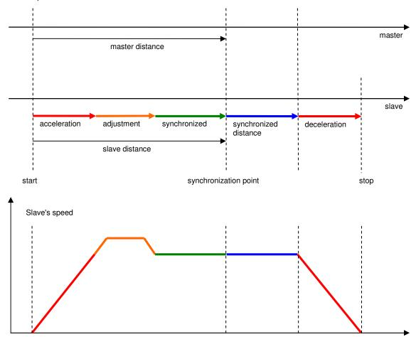
After adjustment, the slave is synchronized in the same phase with the master. The master distance and the slave distance must be defined in so that the slave is synchronized before the synchronization point.
