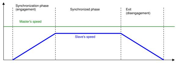
The slave ramps up to the ratio of the master velocity and locks in when the master's speed is reached. Any lost distance during synchronization is not caught up.
