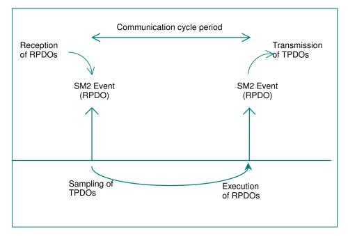
In this synchronisation type, the EtherCAT® master is supposed to embed TPDO and RPDO in the same EtherCAT® telegram.
