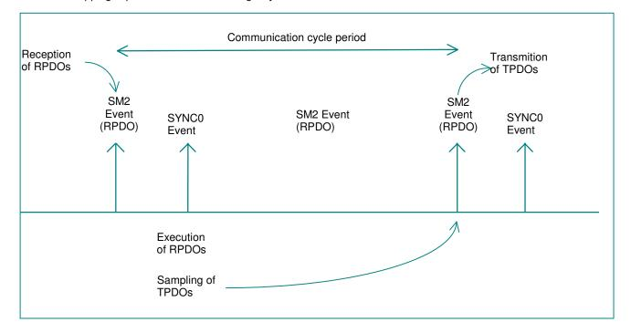
In this synchronisation type, the EtherCAT® master is also supposed to embed TPDO and RPDO in the same EtherCAT® telegram.
