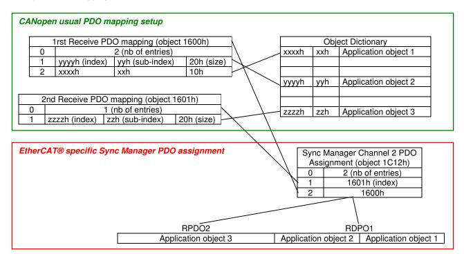
These setups can be performed by using the SDO communication channels either with the **Gem Drive Studio** software or with an EtherCAT® master.
