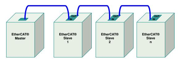
RJ-45 sockets on EtherCAT® slaves are labelled "IN" and "OUT". The EtherCAT® master should be connected to the first EtherCAT® slave using the "IN" RJ-45 socket of the EtherCAT® slave.
