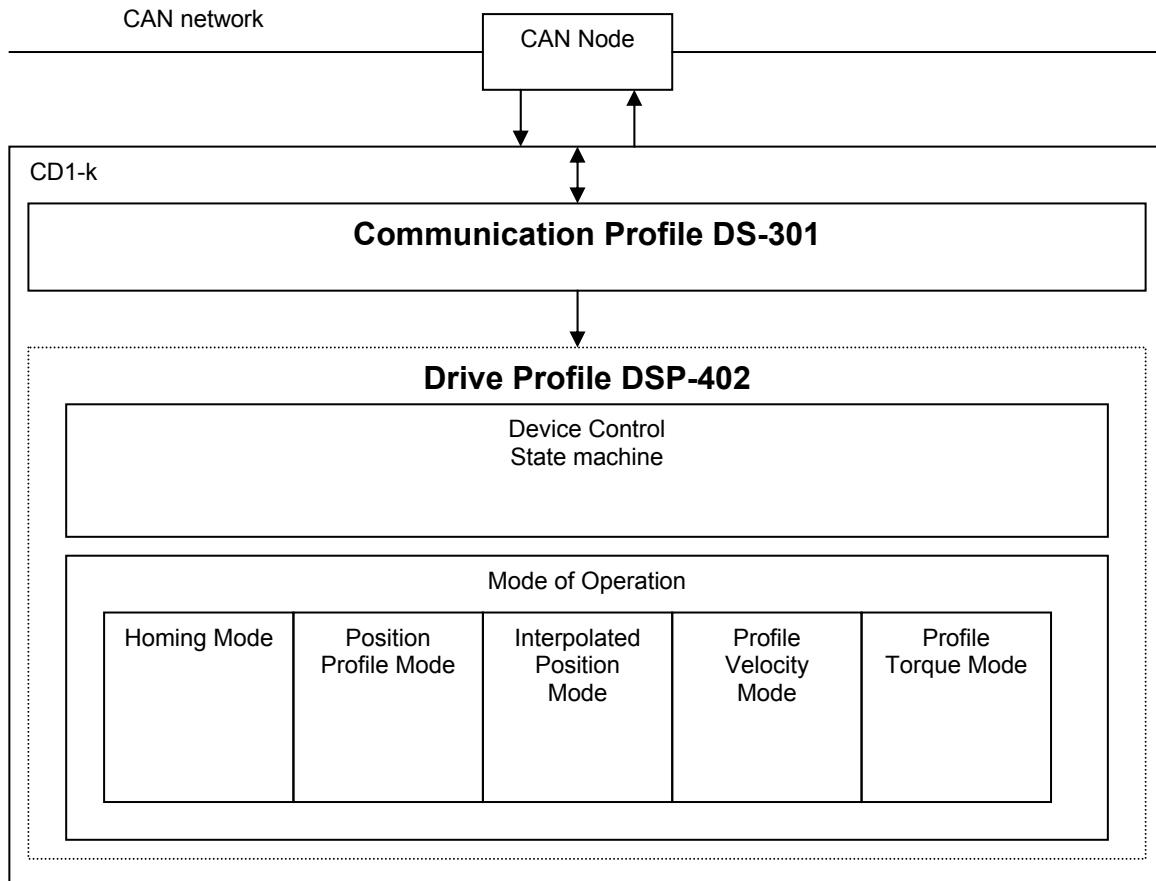
**Device Control:** The drive starting and stopping are executed by the state machine.
