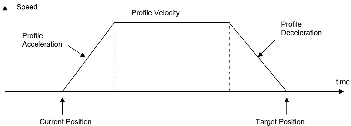
The speed profile is trapezoidal (motion profile type = 0) or S-curve (motion profile type = -1).
