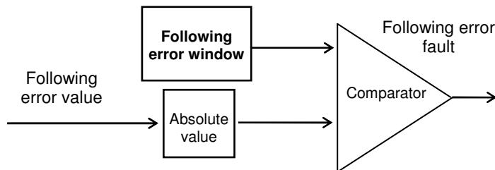
The measured position following error value is continuously compared with the **following error window** parameter value. When the measured position error is exceeding the **following error window**, the position following error fault is released.
