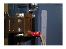
Make the shield cables out of flat braid. Make the shield wires as short as possible. If there are 2 or 3 P874s/P879s in the system fix a shield cable to each one.
