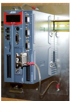
Fix the Shield cable to the D-Type socket fixing screw. Trap the crimp eye between the D-type plug and the hex socket that it screws into. Make sure that the D-Type still makes good contact with the socket. The "eye" must not be too thick; less than 1mm.
