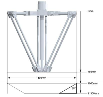
TABLE(100,1100)' Cylinder diameter TABLE(101,(60/360)\* 2\* PI)' Cone angle TABLE(102,400)' Total height TABLE(103,150)' Cone height TABLE(104,0)' X offset TABLE(105,0)' Y offset TABLE(106,750)' Z offset
