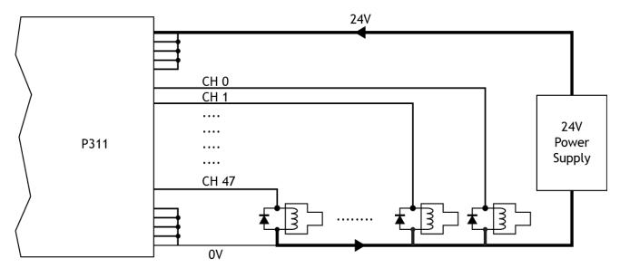
Note that each solenoid coil MUST have a suitable flyback diode across the coil !
