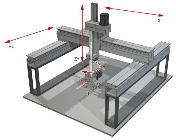
Once the frame is enabled DPOS on the X, Y and Z axis are measured in axis counts. The wrist axis is set to use Nanoradians. You can of course set UNITS for all axis to any suitable scale.
