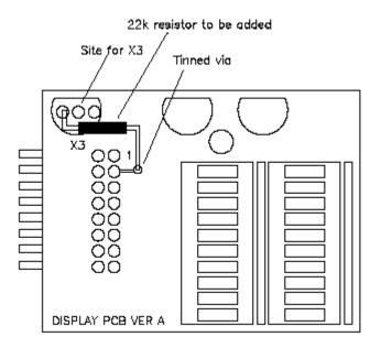
The resistor to be added should be approximately 22k 1/4W or 1/2W type.
