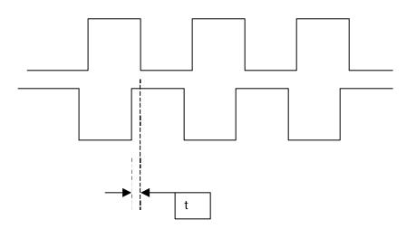
When the A and B pulse trains are not at 90 degrees, the maximum frequency limit is reached when 1/t > 1MHz.
