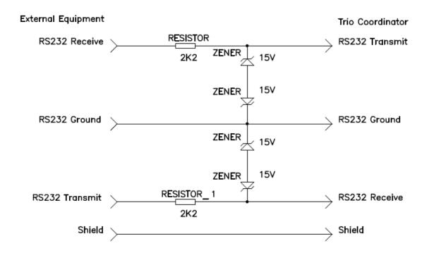
For the RS232 protection to work correctly it must be permanently connected to the controller, so that the zenner diodes are referenced to the controller ground at all times. Because of this you MUST connect the RS232 protection circuit to the controller before connecting the external equipment to the RS232 protection.
