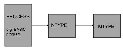
When both MTYPE and NTYPE registers have a move loaded and another move command is issued, this is sent to the PROCESS BUFFER for that particular process in the multi tasking system. Once the process buffer is has a move in it, no more moves can be buffered so if a process issues another move, it will wait until the move in progress has finished so that the buffered moves can all shuffle forward and leave room in the process buffer.
