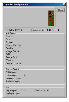
The controller's hardware status can be checked by clicking on the pull-down menu "controller + controller configuration". Information about the axes and I/O that have been recognised by the Motion Coordinator will be displayed in the window. This should agree with the actual configuration of the system.
