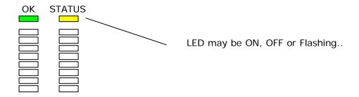
If the OK LED is ON (Green), the Motion Coordinator's processor is working.
