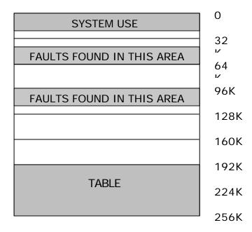
The suspect SRAM device can be identified as U28 on the MC206 PCB. The part number is IS62LV2568LL-70H and the date codes are 0040 and 0049. All MC206
