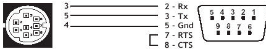
Motion Coordinator to 'AT' style PC with 9pin serial connector
