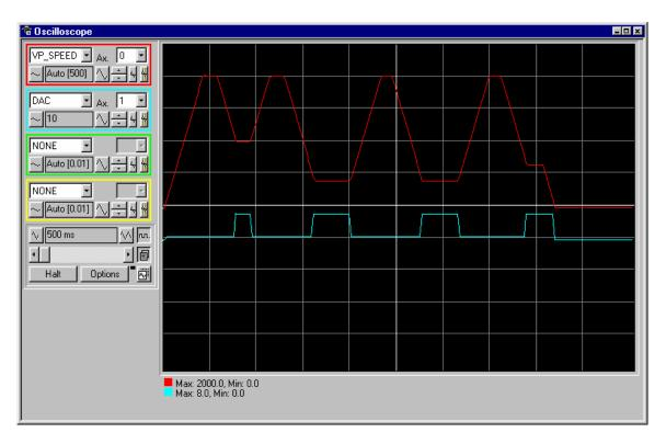
The 'scope trace shows the speed being ramped down firstly from 2000 to 1000, then to 400 and finally to 650 for the MOVECIRCSP. The blue trace shows the MTYPE. This is being copied into the DAC parameter of axis 1 to allow it to be displayed by the 'scope.
