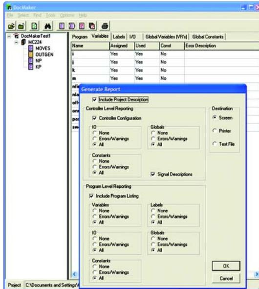
DocMaker analyses the content of the program files in the project. It can be used to print program listings and to report on the programs (variables, labels, I/O and VR's) and on overall I/O and VR usage. There is also a checking routine which does a quick check on the whole project and flags up possible errors
