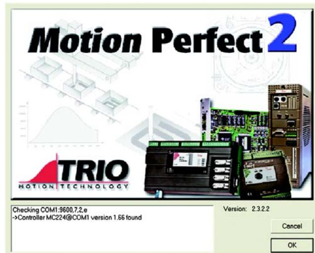
The splash screen features a small messages window (bottom left) which is used to display the status of the connection process. In this example *Motion Perfect* is connected to an MC206X controller via serial port COM1.
