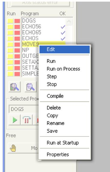
Right clicking on an entry in the program list causes a pop-up menu to appear allowing easy access to operations commonly performed on programs. The right click operation highlights the entry in the program list under the cursor whilst the pop-up menu is visible. It reverts to the program which is currently selected on the controller when the menu is closed.
