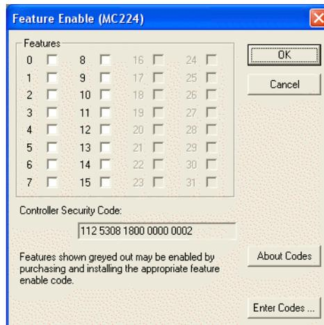
This display shows the features which are currently available. If the codes for additional features have been purchased, the relevant boxes will be available for checking, otherwise the check boxes will be greyed out.
