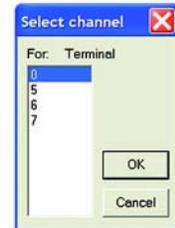
When *Motion Perfect* is in disconnected mode then, on starting the terminal tool you will be presented with a dialog to select the communications port for connection. The available ports will be those previously configured in the communications options tool. Selecting an interface (probably COM1) and pressing "OK" will start a terminal tool. Only one terminal tool can be used at any one time when operating in disconnected mode.
