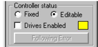
When the controller is fixed into EPROM, the programs actually still run from RAM. The information stored is copied into RAM when the controller is first started, therefore if the controller has been switched off for an extended period, or there is any corruption of the RAM, it will be refreshed with a correct copy of the programs.
