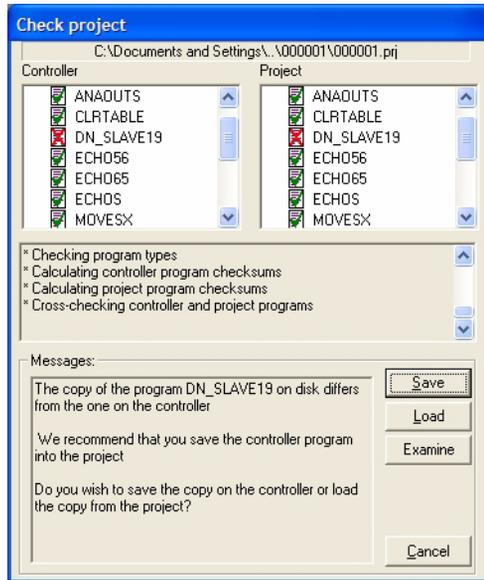
You will need to use your judgment to decide whether the disk or controller version is correct. Typically, if you are recovering the project after a comms failure or PC crash then the version on the controller should be saved. If you have modified the disk based copy of the program then you will need to load this version onto the controller. The examine button starts an external compare program to allow you to visually compare the version on the controller to the one on the PC.
