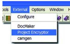
The EXTERNAL menu in *Motion Perfect* allows you to run other programs directly from the main *Motion Perfect* menu. In our example shown here, the menu has been configured to launch two other Trio applications, CAD2Motion and DocMaker. Further information on these applications is given at the end of this chapter.
