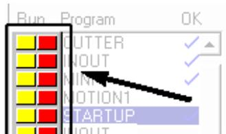
The run buttons provide short cut keys for running, stopping and single stepping programs. They can be in one of three states, red, green or yellow.
