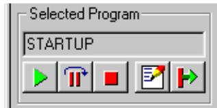
The text box displays the currently selected program and the buttons below, the operations which can be performed on that program.
