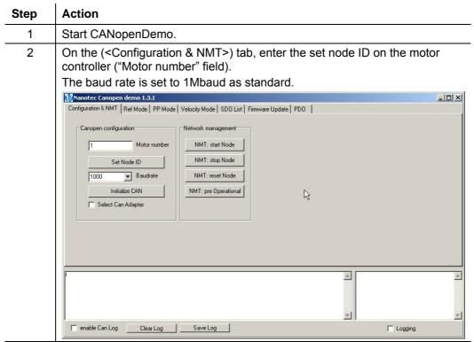
Press the <Initialize CAN> button to accept the node ID and to initialize the CAN device (e.g. PCI board).
